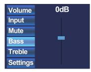
The other settings which can be changed to the zone is the two band tone control. The tone control can be activated by selecting the 'Bass' and 'Treble' buttons, and the adjustment of the tone control works with a fader just as the volume control. You can increase and decrease the high and low tones the same way as adjusting the volume, by simply rotating the selection dial. The Bass and Treble both can be adjusted between the ranges of +14dB and -14dB.
