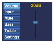
When the desired setting is selected, you can change it by pushing the dial. For example, when Volume is selected, the attenuation on top of the fader will illuminate and the volume can be changed by rotating the dial. When the volume is set to the desired level, press the dial again for scrolling between the settings. You can select the input source by rotating the dial till 'Input' illuminates.
