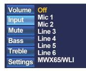
When 'Input' is lit, you can push this button and you will be redirected to the input selection window. This window shows all (configured) input channels which can be selected. You can scroll through the inputs by rotating the selection dial, and the desired input can be selected by pushing the dial.
