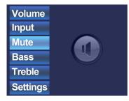
When the input selection is made, you can scroll further through the menu and make other changes such as muting, and changing the tone control. When the zone should be muted, just scroll to the 'Mute button' and push the selection dial. When the selection dial is pushed, you can toggle between 'Mute' and 'Unmute'.
