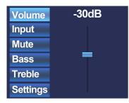
The main screen provides an overview of the functions which can be controlled for the zone it is connected and configured to. Settings such as Volume control, Input signal selection, Mute and Tone control can be made for the corresponding zone. On the left side of the display are all the possible settings displayed, and scrolling between the settings can be done by rotating the selection dial. The settings will illuminate one by one, when rotating the dial.
