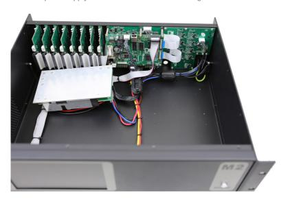
**Step 4:**Connect one side of the supplied flatcable to the connector P1 of the DSP board.
