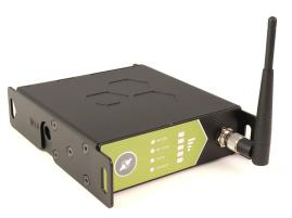
Luna is the essential flex unit that gets the job done, being able to transmit DMX or receive DMX/RDM for one universe. Featuring the same reliable CRMX as all other devices from LumenRadio it also features Bluetooth connectivity in a compact and rugged format.
