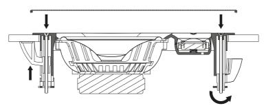
6) After the screws are tightened and the speaker is level with the surface, the front grill can be assembled to the loudspeaker.
