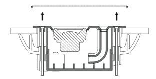
4) Connect the loudspeaker connection cable to the gold plated spring clamp connectors. Press the button of the corresponding terminal down and insert the connection cable. After releasing the button, the cable is connected to the loudspeaker. The Red terminal indicates positive (+) pole and the Black terminal indicates the negative (–) pole.
