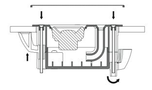
6) After the screws are tightened and the speaker is level with the surface, the front grill can be assembled to the loudspeaker.
