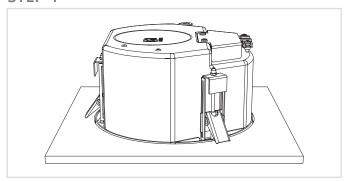
Fix the speaker in the provided opening by tightening the screws of the mounting clamps using a screw driver.
