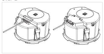
Remove the cover and connect the cables to the ceramic connection terminal by inserting the cable in the corresponding hole and tightening the screw. The remaining two terminals can be used to link through to other speakers.
