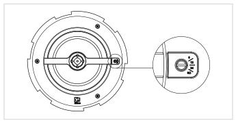
Using a flat head screwdriver, the power tap or low impedance selection can be made.
