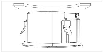
Make sure the spacing between the mouting surface and the clamp is bigger than the thickness of your ceiling plate. Insert the speaker until the clamps snap in place
