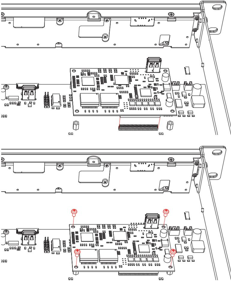
Once inserted and positioned correctly, the ANX44 can be secured to the XMP44 by inserting the 4 original screws (removed in step 3) to the M3 spacers.
