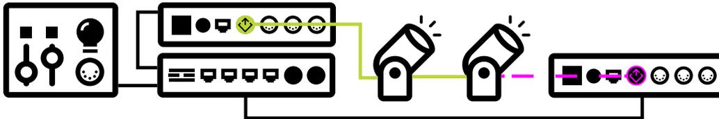
Once a link in the DMX chain gets broken or disconnected the slave port will start outputting DMX and the lights will continue to operate as expected. As soon as the broken link is restored the redundant port will go back to an idle state.
