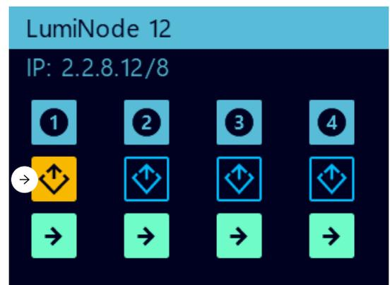
In order to clear warnings, scroll to the following display and press the jog wheel. This screen can be found when scrolling left once when ports 1-4 are shown or to scroll all the way to past the last detailed port info.
