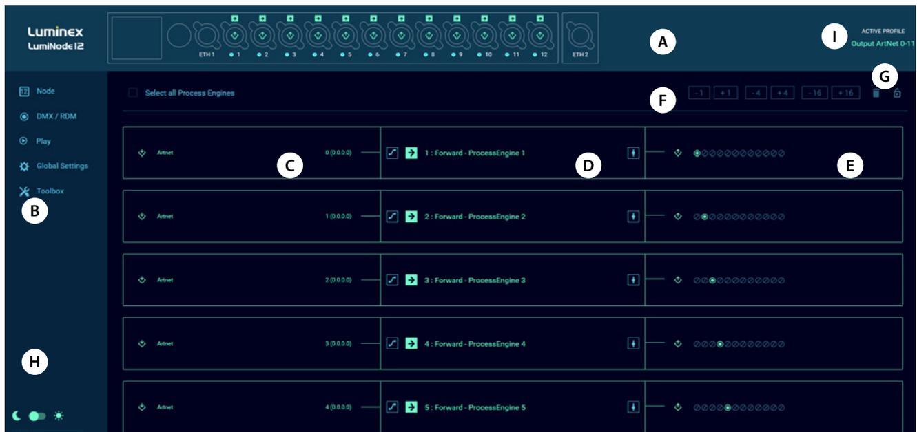
**(A) Image of your LumiNode:** Depending on the model you are using; the image might differ from the one displayed above. This product image shows the configuration of each DMX port. The center icon within each DMX port represents an input or an output. On the top of each port, you can see the mode of the Process engine linked to that port.
