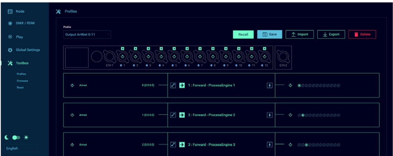
When a profile has been selected the user can scroll down to the bottom of the profile preview to see the IP settings in this profile. By default, the LumiNode will NOT load the IP settings that are
