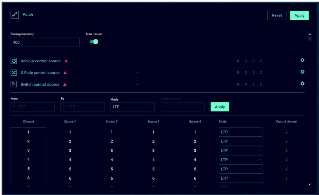
From this panel, you can define the complete patch per source, with any merging policy, or control source.
