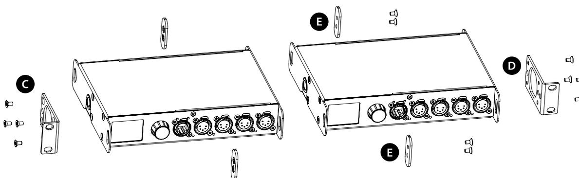
To combine a LumiNode 4 device with a Luminex half 19" device, style GigaCore 10, the mounting procedure differs a little. The bolt (F), not included, replaces the rear couplers at the rear side of the device. Use the correct bolt, M10x20, with a screw wire no longer as 20mm. You can order this part from Luminex (Part Number: R 90 01042)
