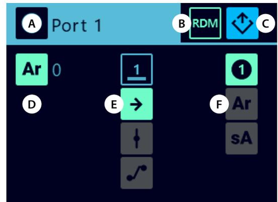
If the lost stream is recovered the LCD display will show this by changing the Output (D) Orange. This way the user can see the stream has been lost
