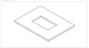
Cut a hole on the desired mounting location. Make sure the dimensions are matching the cut-out measurement for the installing in-table mount box.
