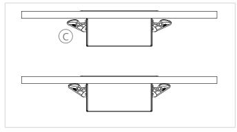
Tightening the bolt will press the clamps against the mounting surface and secure the in-table mounting box in place.
