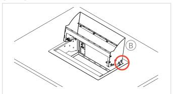
After installing your desired CASY modules, the module insert can be mounted in the box.
