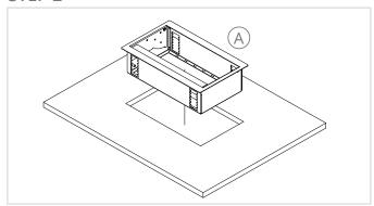
Place the in-table mount box in the cut-out, making sure it is facing the right direction. It can be mounted in surfaces with a thickness ranging from 6 to 50 mm.
