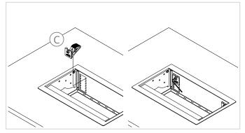
Secure the in-table mounting box in place by installing the BlindSnap $^{\text{TM}}$  clamp and tightening the bolt using the included Allen key.
