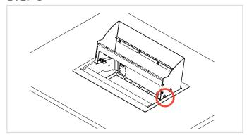
Another set of spring loaded pins keeps the lid from closing, push in these pins and close the lid until the next set of pins touches the box.
