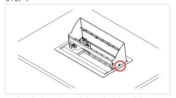
Push in the last pins and close the lid until these pins snap in place.
