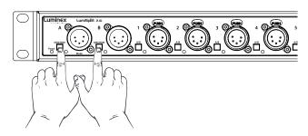
Step 2: Press the output button corresponding to the desired mode. A list of the different modes can be found on the label on the rear of the device.
