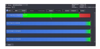
The temperature sensor will indicate the actual inner temperature of the LumiSplit. The contact sensors will display the status of all DC/DC converters. A DC/DC converter's sensor with a value of 1 means the DC/DC converter is working correctly.
