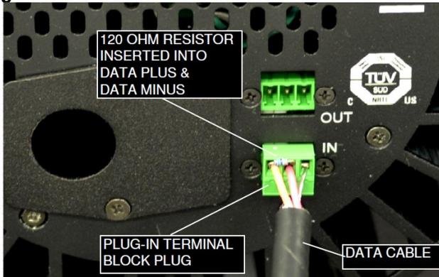
**Figure 6 Data Cable Termination**
