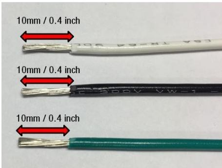
**Stripping Wire:** Remove a minimum of 10mm / 0.4 inch insulation off the 14 gauge wire before inserting into the phoenix connector.
