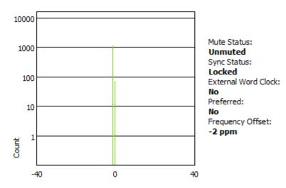
A histogram that shows a distributed range of offsets indicates an unstable clock - it is having to change its offset significantly, and often, to stay in sync with the master clock. This can be due to overloaded network links, or poorly-implemented EEE. A device in this state is highly likely to lose sync with the master clock.
