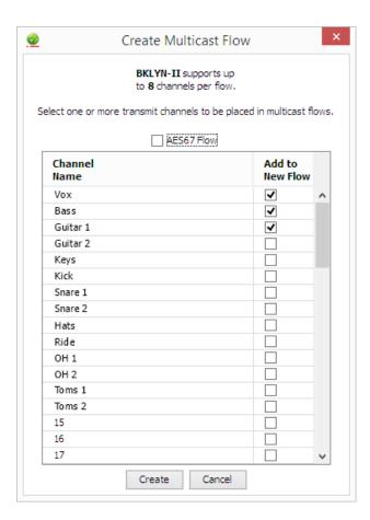
The window shows a list of the Tx channels for the device, and allows you to add them to the new multicast flow that is being created, by checking the tick box next to each channel name. Once you have selected all the channels required, create the multicast flow by clicking the **Create** button at the bottom of the dialog box. To abandon creating a new multicast flow, click **Cancel**.
