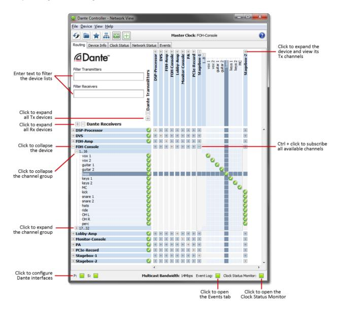
The Rx channels associated with any device can be displayed by clicking on the [+] to the left of the device name in the left-hand column of the grid. The Tx channels associated with any device can be displayed by clicking on the [+] above the device name on the top row of the grid. When this action is performed the grid view expands to show each channel of the device, and the [+] becomes a [-]. Clicking on [-] collapses the view. You can also group channels into sets of 16.
