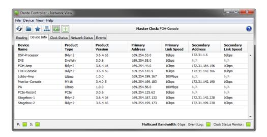
The Device Info tab provides a network-wide overview of device configuration and operating information.
