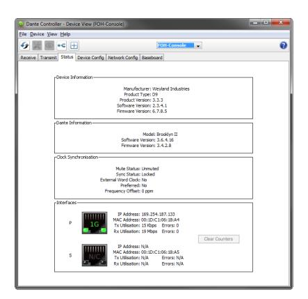
The tab is divided into sections. The information presented on this tab can be very useful when investigating networking or clocking issues in the system. The Refresh button can be used to update this information if required.
