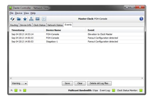
The Events tab provides information on significant changes and failures in the network.
