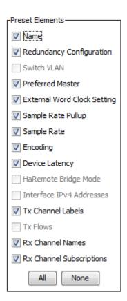
If the target network is not identical to the original network (from which the preset was saved), some elements might not be applied successfully. For example, if some devices on the target network do not support the same range of sample rates as the devices on the original network, you could choose not to apply the 'Device Sample Rate' element, and change the sample rates manually instead, once the preset has been applied.
