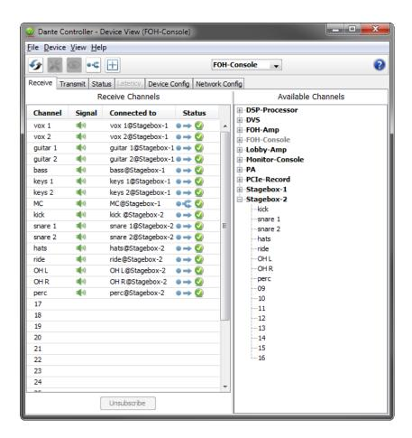
The tab is split into two panes: Receive Channels, and Available Channels.
