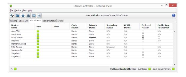
The Clock Status tab provides a network-wide overview of the clocking state within the network.
