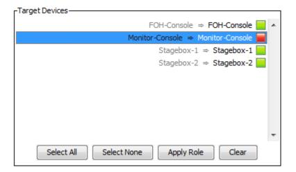
The LED icons against each device indicate the assignment status of the device.
