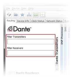
The filtering is case-insensitive. For example, in the Dante Controller Network view shown here, entering the string "foh" in either of the Filter fields would display only the FOH-Amp and FOH-Console devices, and their channels.
