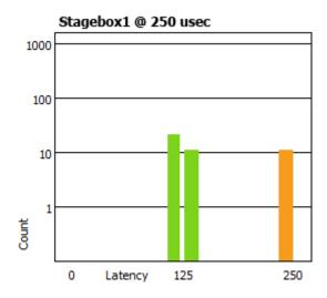
If any bars are red, it indicates lost packets, and audio loss. The receiver latency should be increased, or the network reconfigured.
