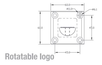
Depending on the mounting direction of the loudspeaker (either horzontally or vertically), the logo on the front grill of the loudspeaker that is held in place by a spring loaded mechanism can be rotated into the direction the speaker is mounted.
